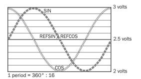
Access to the process data used for speed control, i.e. to the sine and cosine signals, is practically always "online". When the supply voltage is applied, the speed controller has access to this information at any time.
