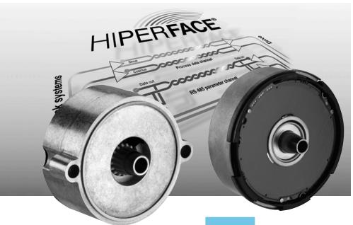
The holistic scanning almost completely compensates for eccentricity errors. The capacitive operating principle can function without ball bearings and is therefore extremely robust. By dispensing with wearing parts, possible error sources are largely excluded, and the motor feedback systems have a high temperature resistance previously reserved for resolvers. Moreover, the system construction allows extremely low power consumption.
